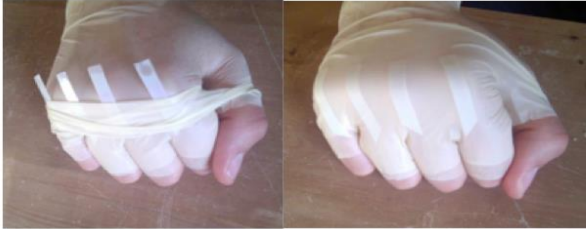
Figure 1 – The placement of the pressure film over the extensor tendon at the MCP joint, before wrapping of the hands with a competition wrap
