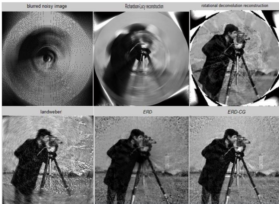
Fig 11. De-blurred image by Lucy-Richardson, RD, Landweber, ERD and ERD-CG methods with rotation of angle degree and 2% of noise[15].
