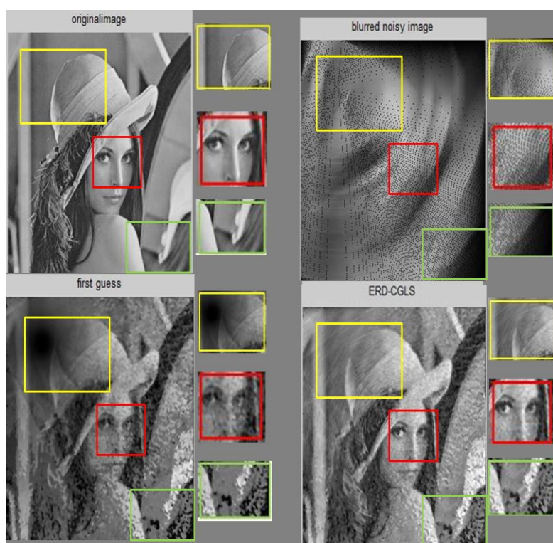
Fig 7. De-blurred image by ERD and ERD-CGLS methods with rotation of angle 20 degree and 2% of noise, the rotating center, doesn't coincide with the image's center[15].
