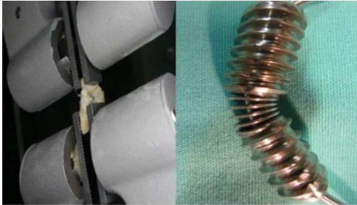
Fig 2a.Uniaxial tension of SLIL Fig 2b.FS in bending and rotating. A k-wire inserted through the cannula.
