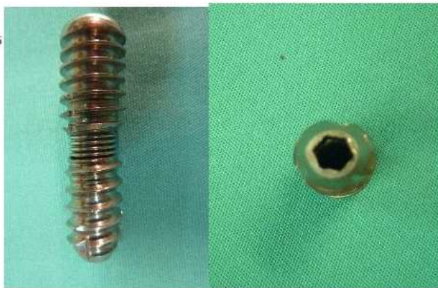
Fig 1c. Cross-section of the cannulated hexagonal shape
