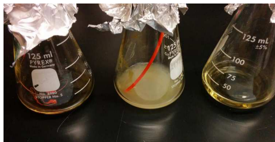
Figure 2. Growth after 96 hours at 37°C in a shaking incubator. The leftmost beaker contains LB media inoculated with PLA plastic extruded from the printer nozzle at 220°C. The center beaker contains LB media inoculated with a segment of unextruded PLA plastic filament from the same spool. The rightmost beaker contains uninoculated LB.
