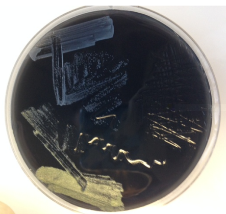
Figure 9. 10 \mu l of each AYE tube (positive control, PLA plastic and negative control) was struck out on Charcoal Yeast Extract solid media and incubated at 37C to grow for 24 hours. Growth revealed that the PLA test part (top, white) appeared to contain a different bacterial species than the positive control tube (bottom, yellow). The negative control was plated on the right (no growth). Under light microscope, both bacterial growths appear coccoid, with the yellow colonies forming clumps more often. Experiment was repeated with parts from UC Davis and Michigan State, plus controls. Contamination was not observed.
