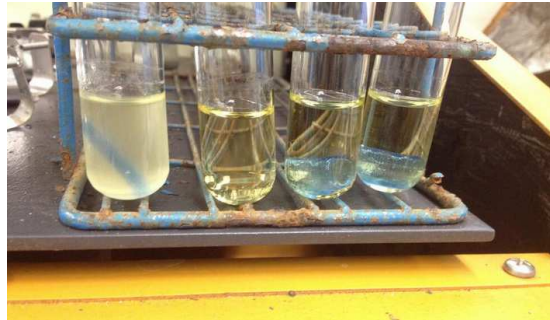
Figure 6. After 48 hours, only the positive control (left) was contaminated. Printed cylinders in LB did not appear to contaminate media.
