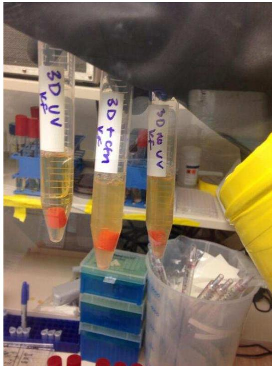
**Figure 8.** After two weeks in anaerobic chamber at 37C in “meat broth,” a non-UV treated part from UC Davis exhibited evidence of growth. All other parts were limp, aside from the positive control. Contaminated media was plated on BHI+blood agar overnight (see Figure 9), and 16S rRNA sequencing was performed on resulting colonies.
