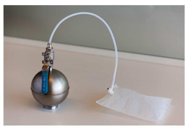
Olfactory threshold testing using the Scentroid SM110C olfactometer and SK5 n-butanol Sensitivity Kit.
