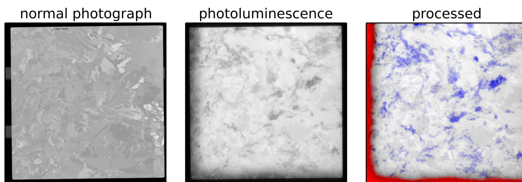
Figure 4. Left: An image of an as-cut silicon wafer before it has been processed into a solar cell. Center: A PL image of the same wafer. Wafer defects, which have a negative impact solar cell efficiency, are visible as dark regions. Right: Image processing results. Defects in the crystal growth (dislocations) are colored blue, while red indicates the presence of impurities.
