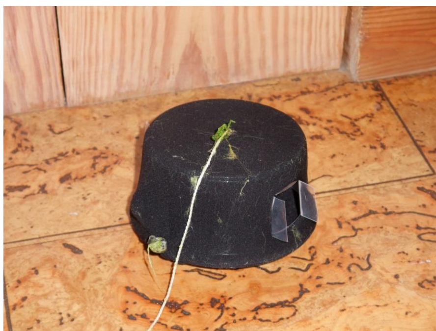
Figure 1. “Feeding station” after use in field trials. Cotton thread attached at the top assisted in positioning and retrieval of stations and to the right is an entrance hole with “doors” intact to ensure opening was not blocked by straying material. A similar opening is found on the opposite side of the station.
