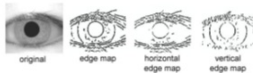
Figure 3. Iris segmentation using Hough transformation.
