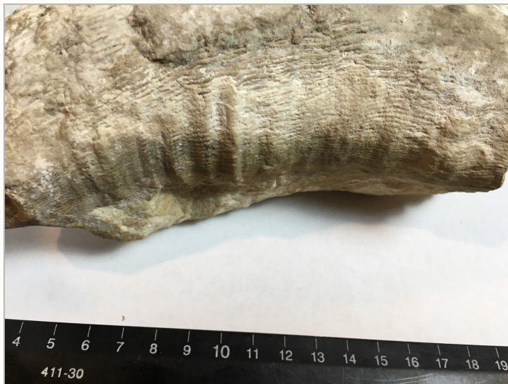
Figure 3: showing the bands on the concave side of the specimen (17 bands in total)
