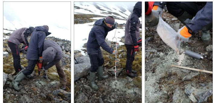
Figure 2. Installation of 1.5 m long thermistors string connected to mini datalogger (site TM13, see in Fig. 1, photographs: P. Tábořík).
