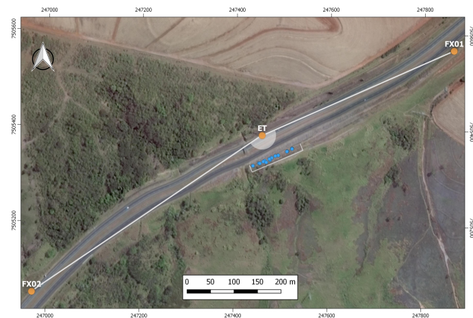
Figure 1. Positioning of the total station (ET), fixed points (FX01 and FX02) and targets distributed on the outcrop surface (blue points).
