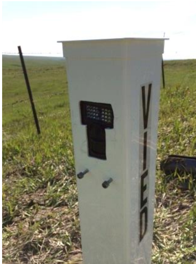
Figure 1: Camera cover showing bolts that form camera platform, hole for camera lens and vinyl decals added for camouflage.
