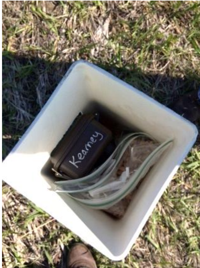
Figure 2: Camera inside cover with sealed bags of beans holding camera in position.
