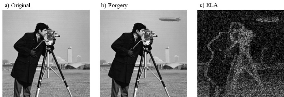
Figure 2. Figure a) shows the original cameraman image, b) shows the forgery, with a zppelin in the background and c) shows ELA for the doctored image.
