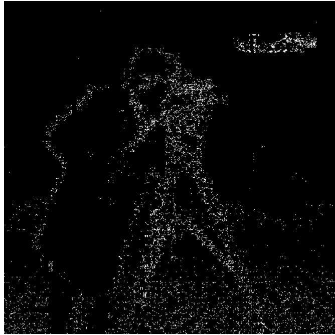
Figure 7. The cameraman image has been wavelet thresholded with a k scale of 4.
