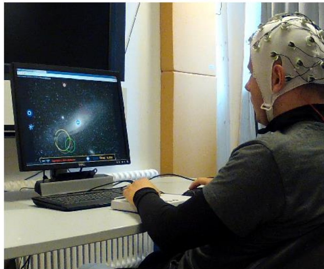
Figure 1. Experimental set up. Participants were requested to perform a secondary oddball task while playing a game as a primary task while EEG signals were recorded.
