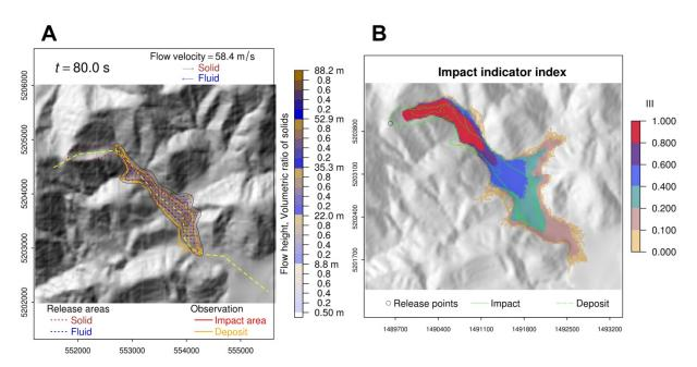
Fig. 1. Results yielded for the Acheron rock avalanche, New Zealand. A: Flow depth after 80 seconds derived with r.avaflow. B: Impact indicator index (III) yielded with r.randomwalk, applying the optimized parameter sub-space.
