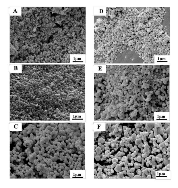
**Figure 1 SEM images of silver nanoparticles on a glass slide after incubation at different temperature and time combinations.** SEM images of AgNPs were obtained at (A) 100 °C for 6 h, (B) 150 °C for 6 h, (C) 200 °C for 6 h, (D) 100 °C for 12 h, (E) 150 °C for 12 h and (F) 200 °C for 12 h.
