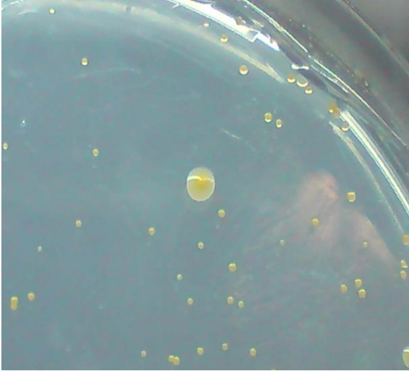
Figure 14: Growth of microorganisms from tap water on formulated colourless agar with 1 g/L yeast extract after 7 days of incubation at 37 °C. Photo of agar plate with close-up pictures of the same plate.
