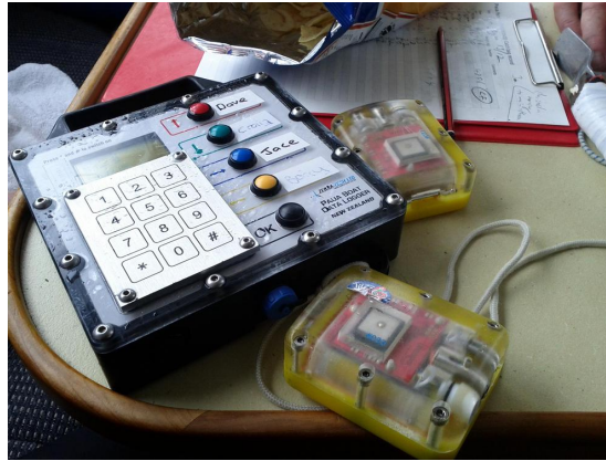
Figure 1. Data loggers used in the current study to record catch and effort data in New Zealand’s abalone (pāua, Haliotis iris ) fishery. The data loggers include a larger boat unit (including buttons for recording catch bags, and a key pad for entering catch weight and other data) and a smaller, dive (or “turtle”) logger that is carried by free divers, and records their position and dive depth (Image by E. Abraham).
