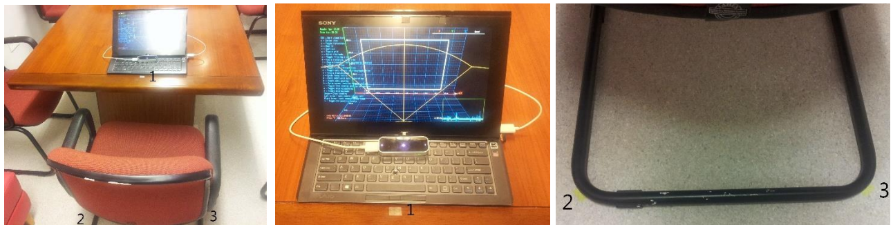
Fig. 1. The setup of the chair, the table, the notebook and the Leap motion controller in the present study. Their positions were all fixed during the whole study.
