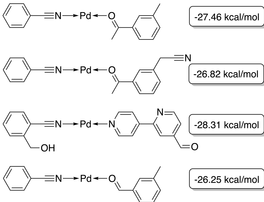
Figure 7 Best-performing individuals of the GBGA with synthetic accessibility constraint after 40 generations. The calculated energy difference is shown to the right of the structure.
