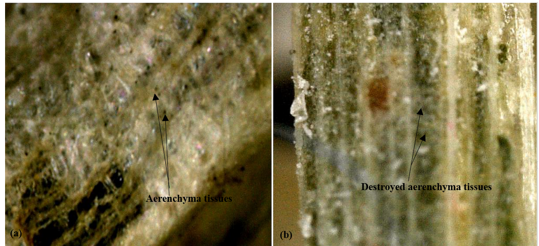
Figure 5 Micrographs (x270) showing aerenchyma tissues in cattail fibers. (A) Untreated; (B) 5% alkali treated.
