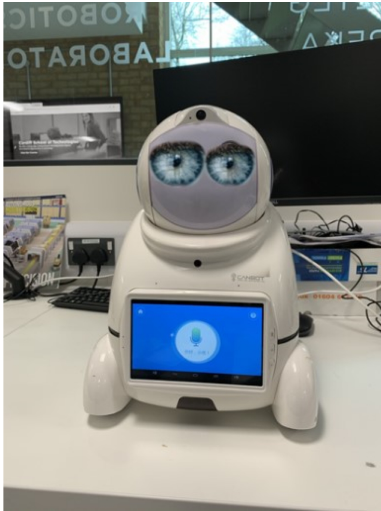
Figure 2 Canbot-U03 robot with human eyes modification.
