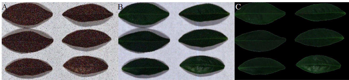
Figure 17 The reconstructed images for the first tea leaf HSI at the sampling rate of 5%. (A) SSCS. (B) BCS. (C) HCSMAROI.
