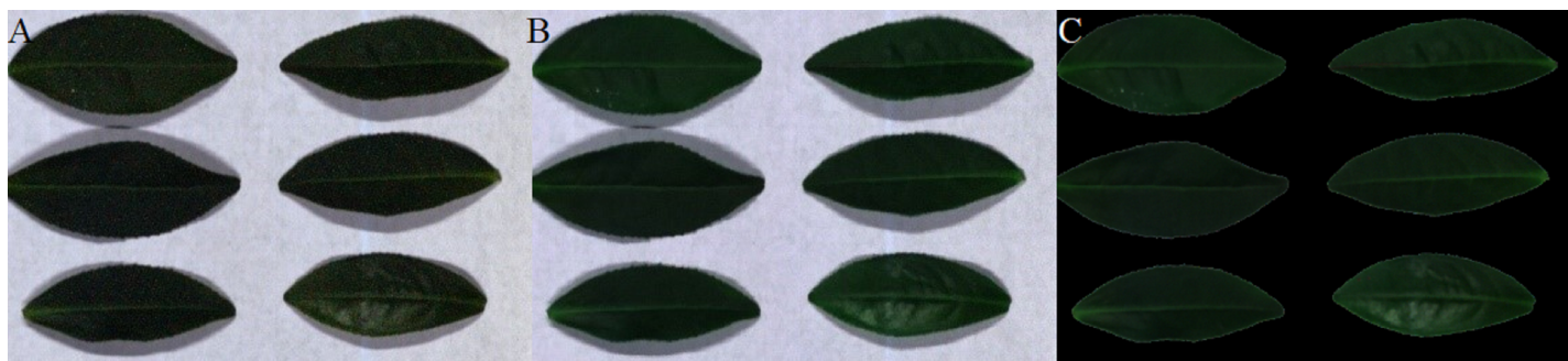
Figure 19 The reconstructed images for the first tea leaf HSI at the sampling rate of 12%. (A) SSCS. (B) BCS. (C) HCSMAROI.
