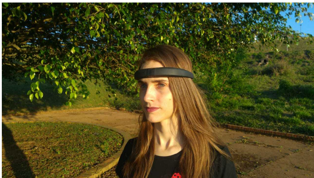
Figure 1 Example of an EEG headband with few electrodes and no need for conductor gel.
