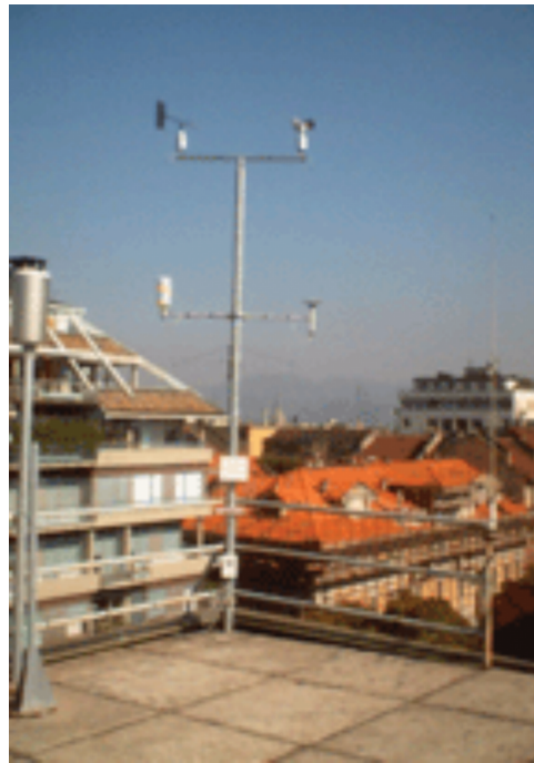
Figure 4 Meteo Weather station at Politecnico Di Torino. The time series data is recorded from the Meteo weather station mounted at the top of DET building and connected with Neuronica Laboratory, Politecnico Di Torino. (Narejo & Pasero, 2017). Full-size DOI: 10.7717/peerj-cs.514/fig-4
