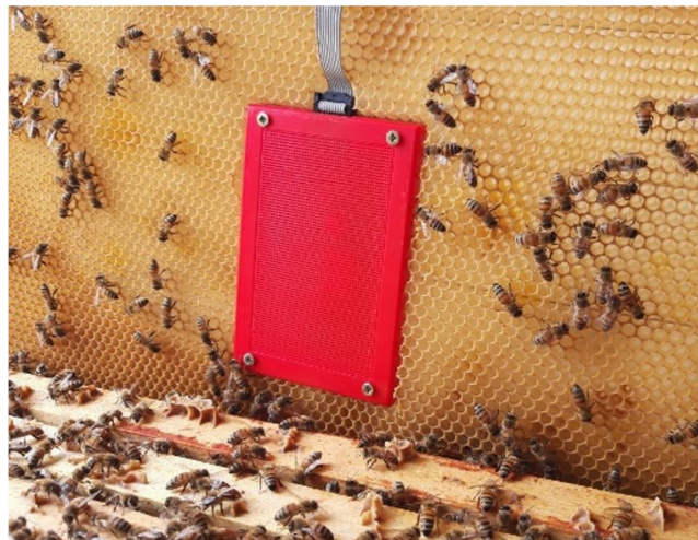
Figure 6 SAMS HIVE sensor frame. Sensors are installed in a 3D printable case placed in a regular brood frame and connected with flat cable to SAMS HIVE device.
