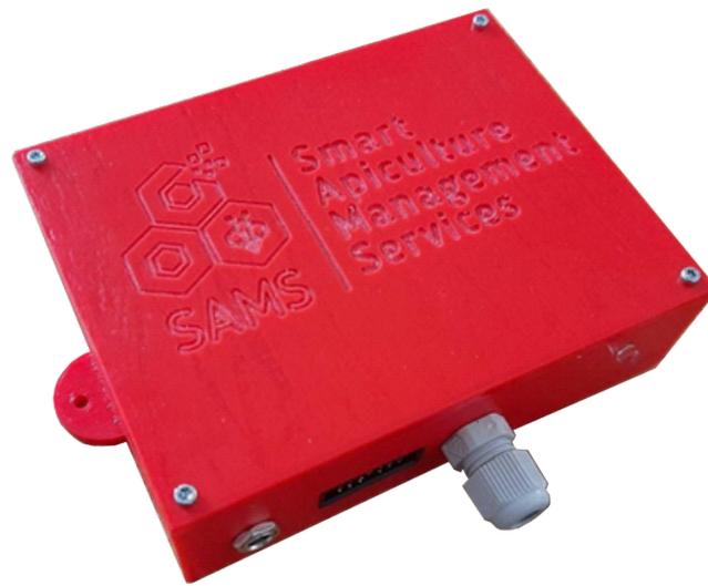
Figure 5 SAMS HIVE case. PCB and components placed in a 3D printable case.
