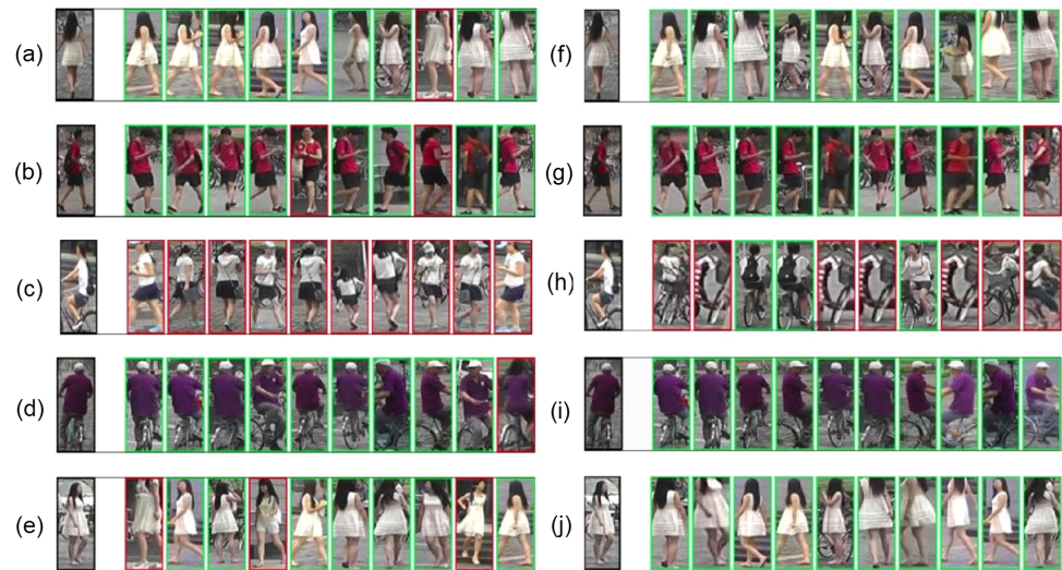
Figure 5 Qualitative results for top 10 close matches of given query images: (A–E) Results of baseline model with standard dropouts; (F–J) Results of proposed ACM based model.
