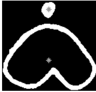
Figure 8 Binary image with the centroid locations superimposed.
