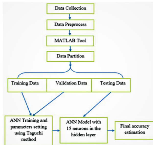
Figure 4 The proposed Improved-ANN (IANN) cancer classification model. It starts by data collection, followed by the preprocess step to clean the data. Then, the data is divided into training, validation, and testing. Then, the ANN is trained and the parameter is optimized using Taguchi method. The final ANN model with 15 neurons in the hidden layer is used to classify the test (unseen) data.
