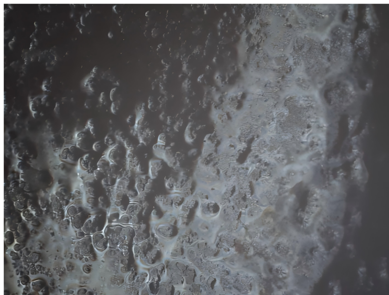
Figure 1 The arrangement of pores on the ceramic surface.
