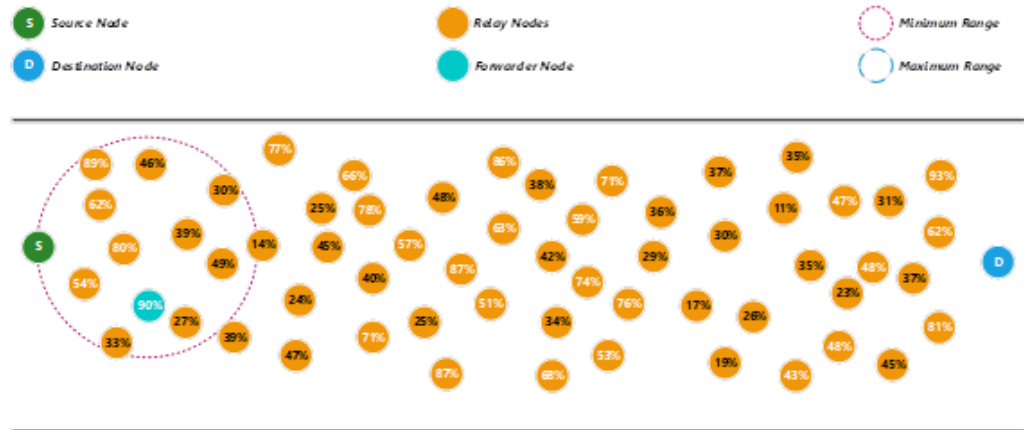
Figure 1 Determine a forwarder node using the minimum range.
