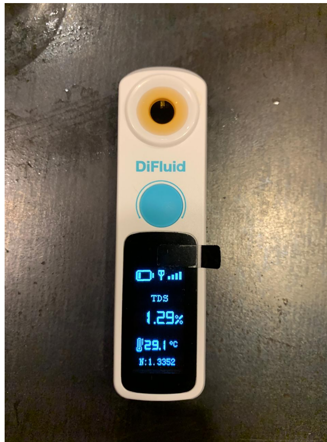
Figure 20 DiFluid device displaying total dissolved solids (TDS) value of 1.29% at a temperature of 29.1 °C, providing coffee quality measurements. Full-size DOI: 10.7717/peerj-cs.3219/fig-20
