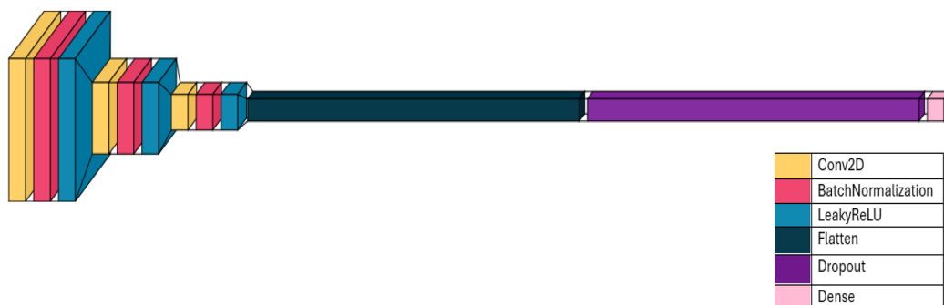
Figure 9 Layer architecture in discriminator network. Full-size DOI: 10.7717/peerj-cs.3167/fig-9
