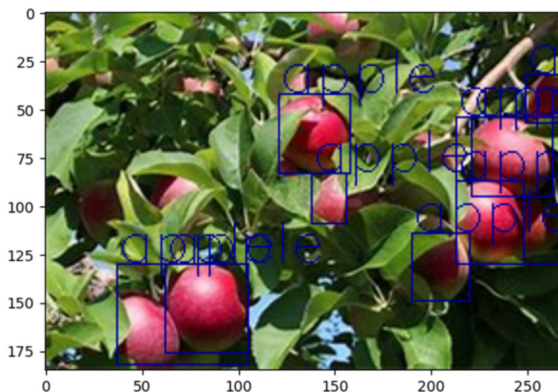
Figure 9 The recognition results of YOLO v8 under close-exposure and closed-conditions.
