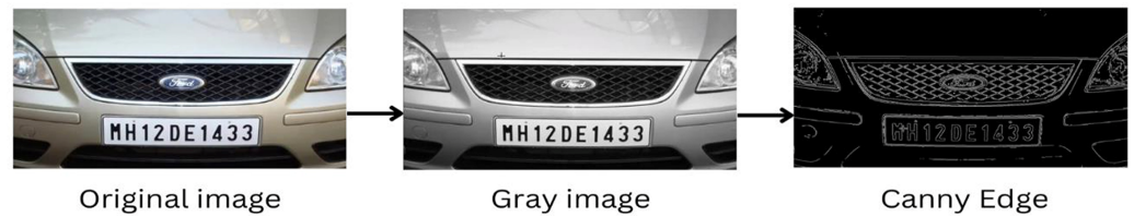
Figure 4 Image conversion for number plate detection.
