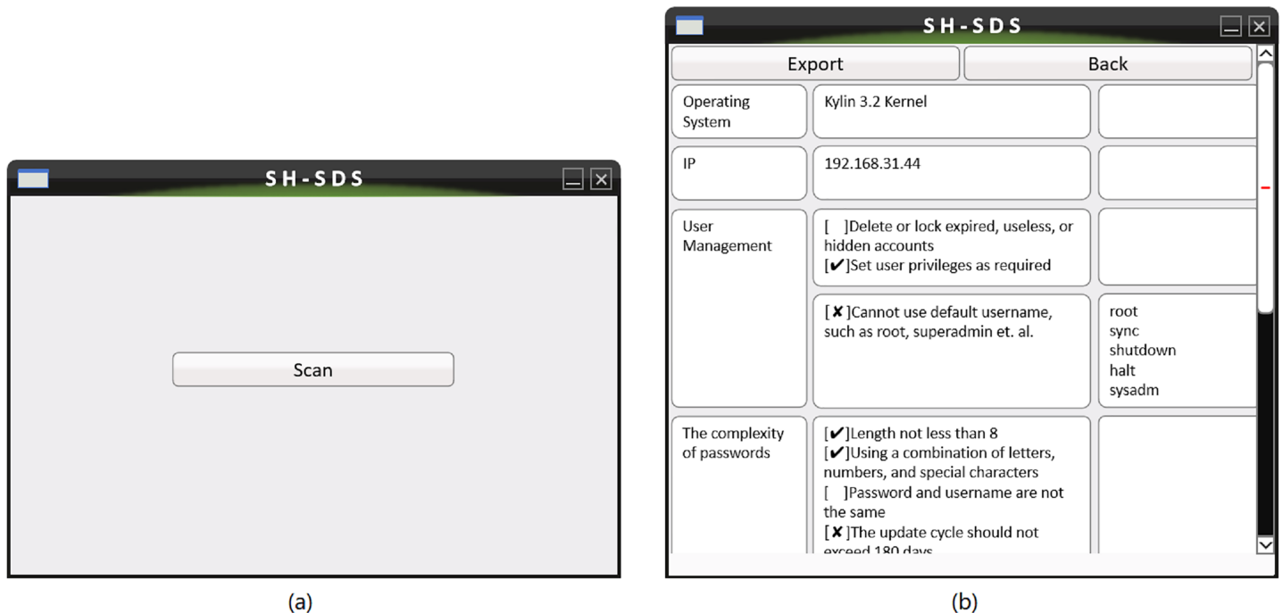
Figure 8 The system's main interface (A) is used to initiate inspection. The system operation interface (B) is used to view and export inspection results.
