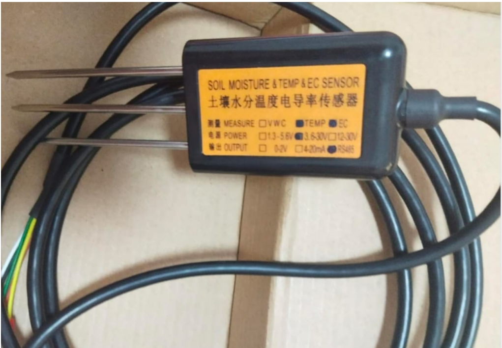
Figure 4 Soil moisture, temperature, and EC sensor.
