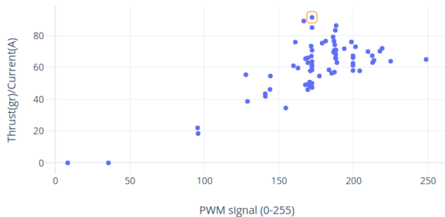
Figure 8 Physical experiment chart, thrust/current vs. rotational speed control signal (PWM signal 0-255).
