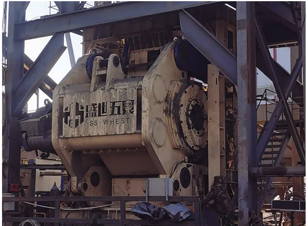
Figure 8 High-pressure roller grinder at the ore beneficiation site.
