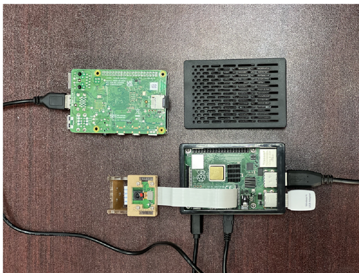
Figure 7 IoT device integration for the proposed model using Raspberry PI 4b model.
