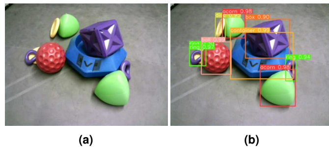
Figure 6. (a) Raw image taken using OpenMV H7 camera at 640x480 resolution of partially occluded VEX game pieces. (b) Predicted object labels using YOLOV8 algorithm and trained weights.
