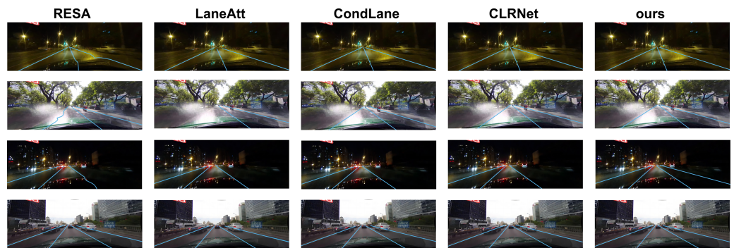
Figure 5 Visualization result of the RESA, LaneAtt, CondLane, CLRNNet, and our method. Image source: CULane dataset, https://xingangpan.github.io/projects/CULane.html .
