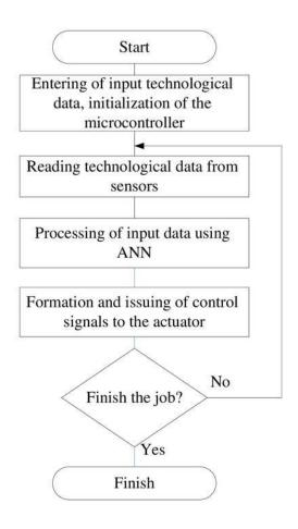
Structural model of the intelligent mini-greenhouse control system in the graph form
