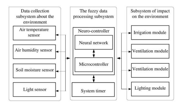
Block diagram of the neuro-controller algorithm for controlling an intelligent minigreenhouse
