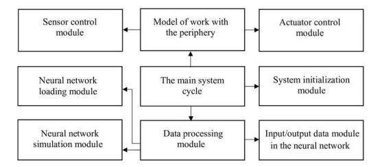
Block diagram of the algorithm of the subprogram for simulating the operation of the neural network
