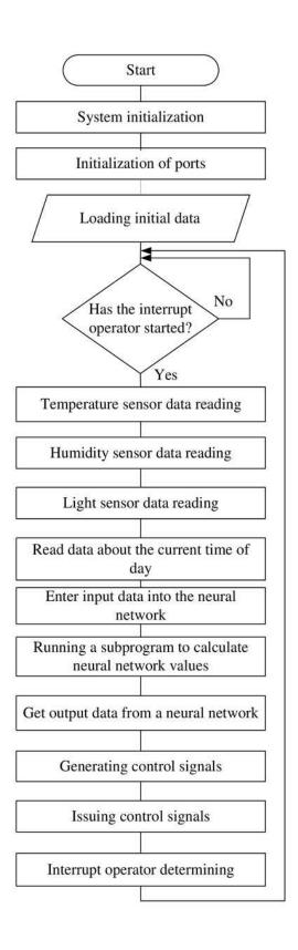
A simplified block diagram of algorithm of neuro-controller operation
