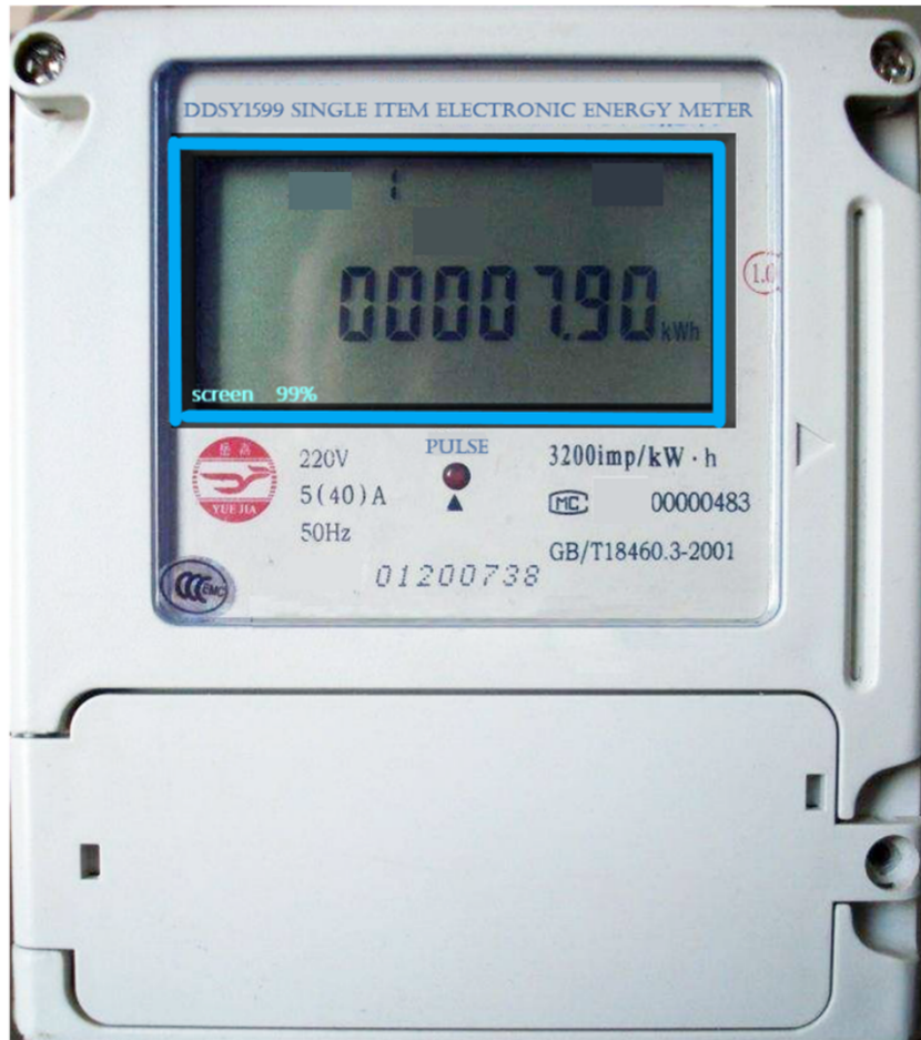
Figure 7 The SSD model detects the effective reading area of the electricity meter. The TensorFlow Object Detection API provides the corresponding eval. py script to verify the trained model. Running the script can verify the test set and generate the corresponding log file. Then, the log file is read through TensorBoard and the verification effect of the model is displayed.
