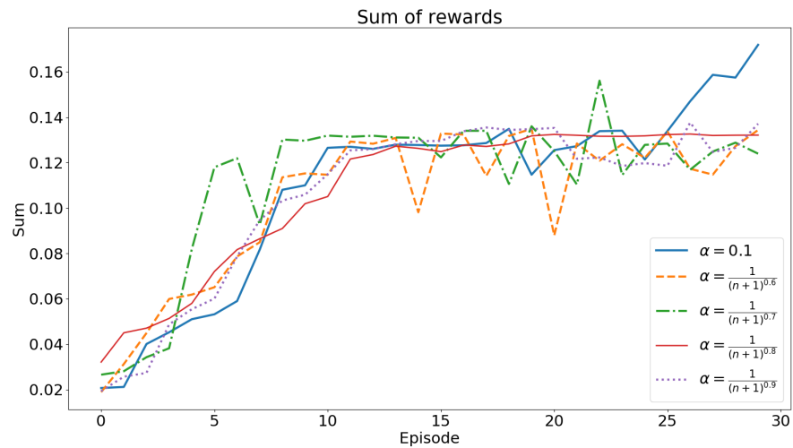
Figure 6 Accumulated rewards for lane changing maneuver. Each curve shows the evolution for a specific value of the \alpha parameter.
