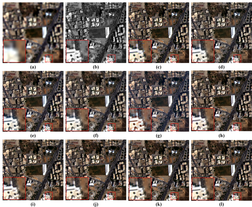
Figure 7 Pan-sharpening results of different methods on a reduced-resolution WV3 testing patch pair. (A) Up-LRMS. (B) PAN. (C) GT. (D) GSA. (E) BDSD. (F) MTF-GLP-FS. (G) TV. (H) PNN. (I) MSDCNN. (J) DR-NET. (K) Zhou et al. (2022) (L) Ours. The photos in this figure are generated from the raw data available at https://github.com/zhysora/PGMAN .
