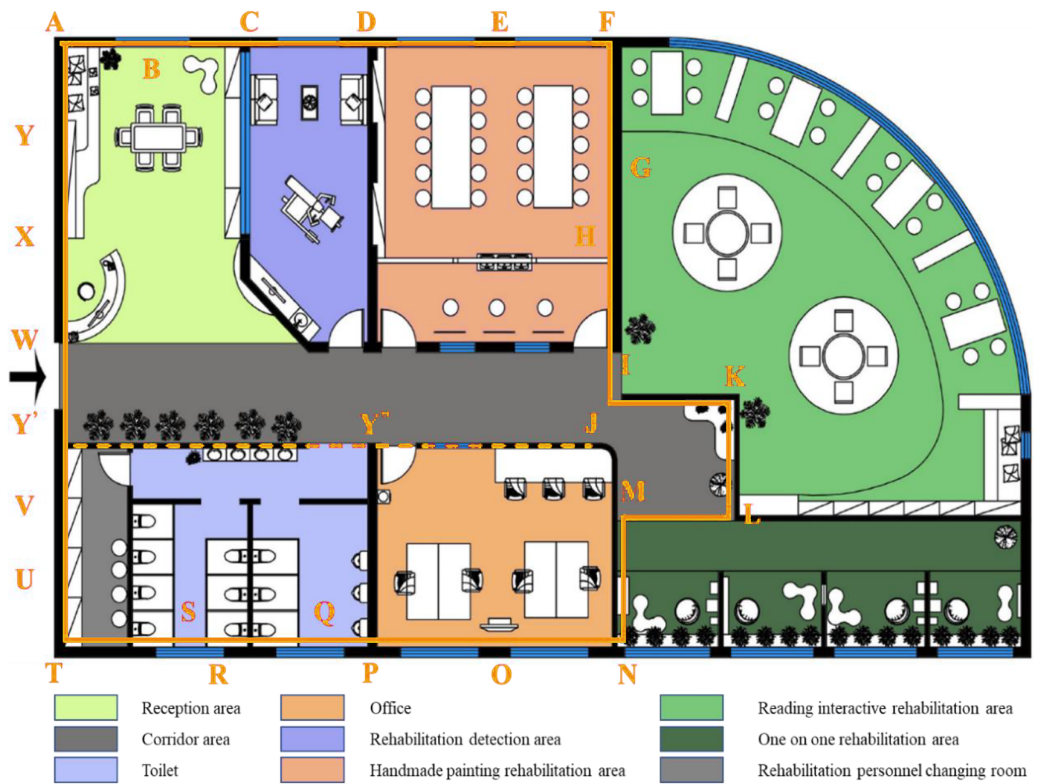
Figure 2 Layout plan of education and rehabilitation space for autistic children. Figure 2 is a top view of the house-type space that has completed the education and rehabilitation of autistic children.
